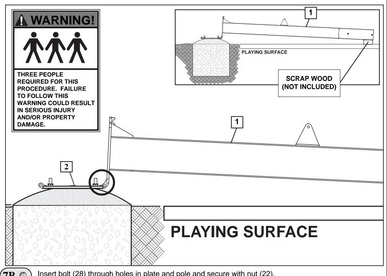
Insert bolt (28) through holes in plate and pole and secure with nut (22). 7B.♀
